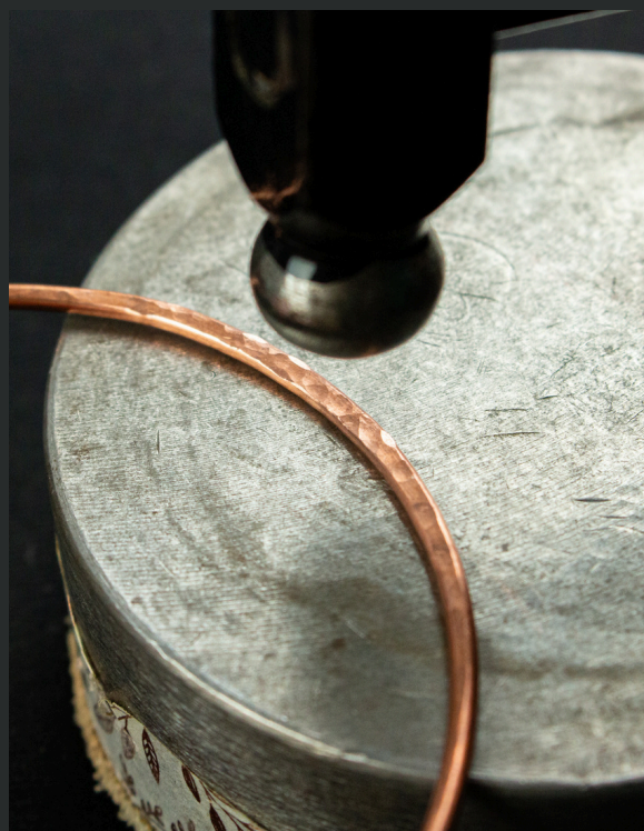
8. When it is done, turn the hammer and use the round end of the hammer to hammer some more to decorate it.
