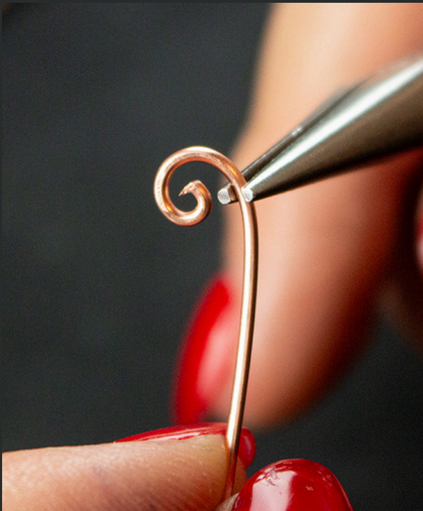
25. Form a spiral at one end with pliers according to the template.
