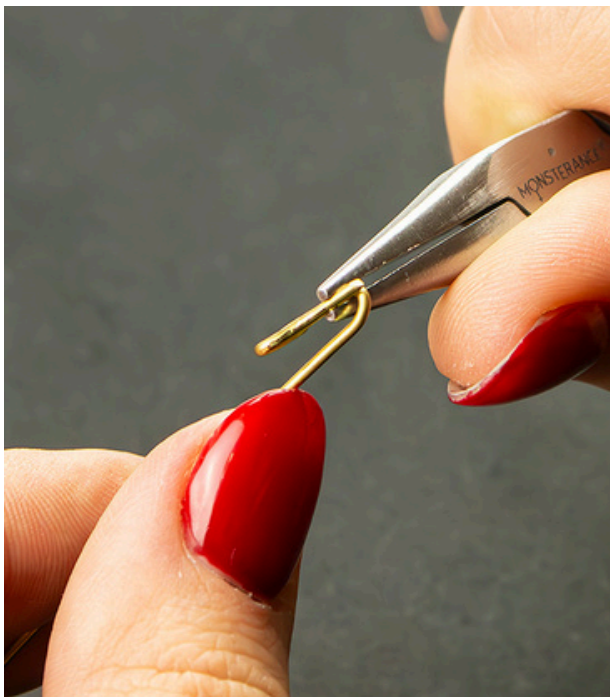
38. Bend the wire back and lead it through the center of the arrow tip.
