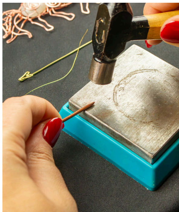
41. Hammer both ends of this wire on an anvil. Hammer about 1 cm from the end, rotating the wire as you work until you achieve a tapered shape on both sides.
