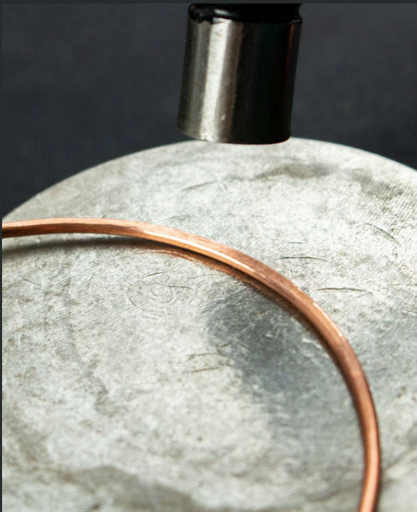
7. Then hammer the loop on the anvil with the flat end of the hammer. Do not hammer the straight ends of the wire.
